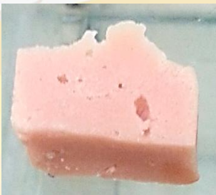
Figure 17: Bubbles are flawed when using the manual method.
