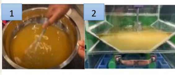
Figure 13: (1) manual mixer method, (2) semi-automatic mixer method
